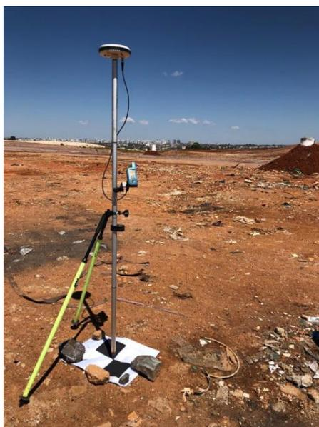
**Figura 3-15 - Base GNSS receptor no Aterro**
