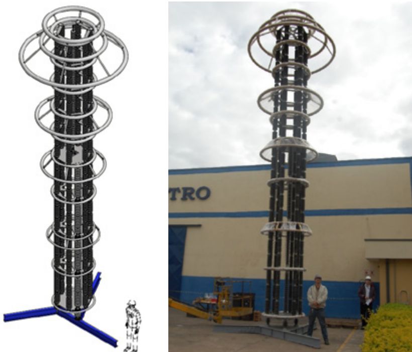
Figure A17.1: Illustration and photo of the project prototype surge arrester
