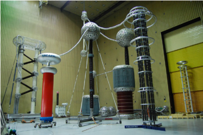
Figure A17.3: UHV surge arrester testing arrangement, with power frequency
