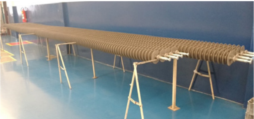
Figure A17.12: Insulator prototypes for the 1,000 kV AC during manufacturing
